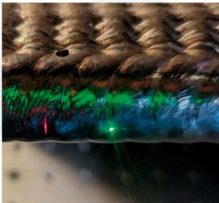
**Above:** Figure 2 A close up of the Ti-alloy sample being scanned by the two lasers of the Adaptive LIPA system, during the adaptive data acquisition
