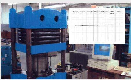
Bearing creep testing and results chart
