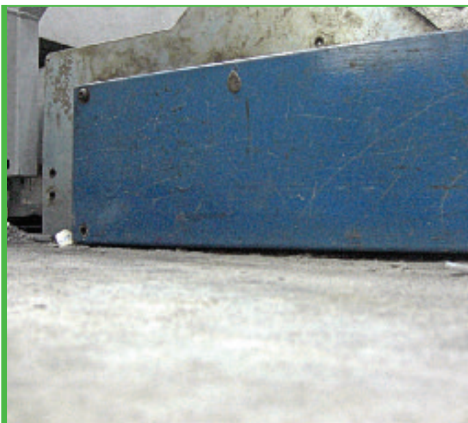
Figure 7. Waste chute panel missing two fixing bolts
