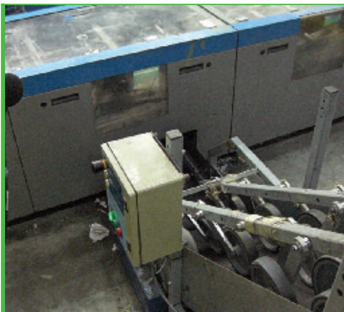
Figure 6. Press waste chute (rattling panel below at ground level beneath control box)
