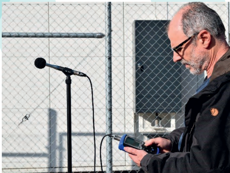
Left: Class 1 and calibrated instruments offer a high degree of precision
