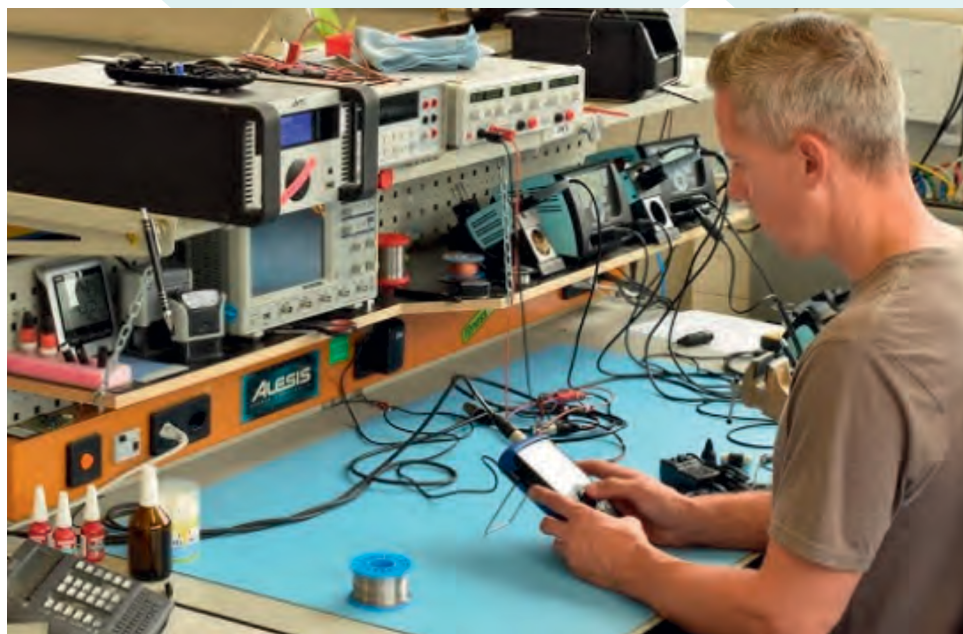
Below: Laboratory calibration in accordance with Part 3 of BS EN 61672
