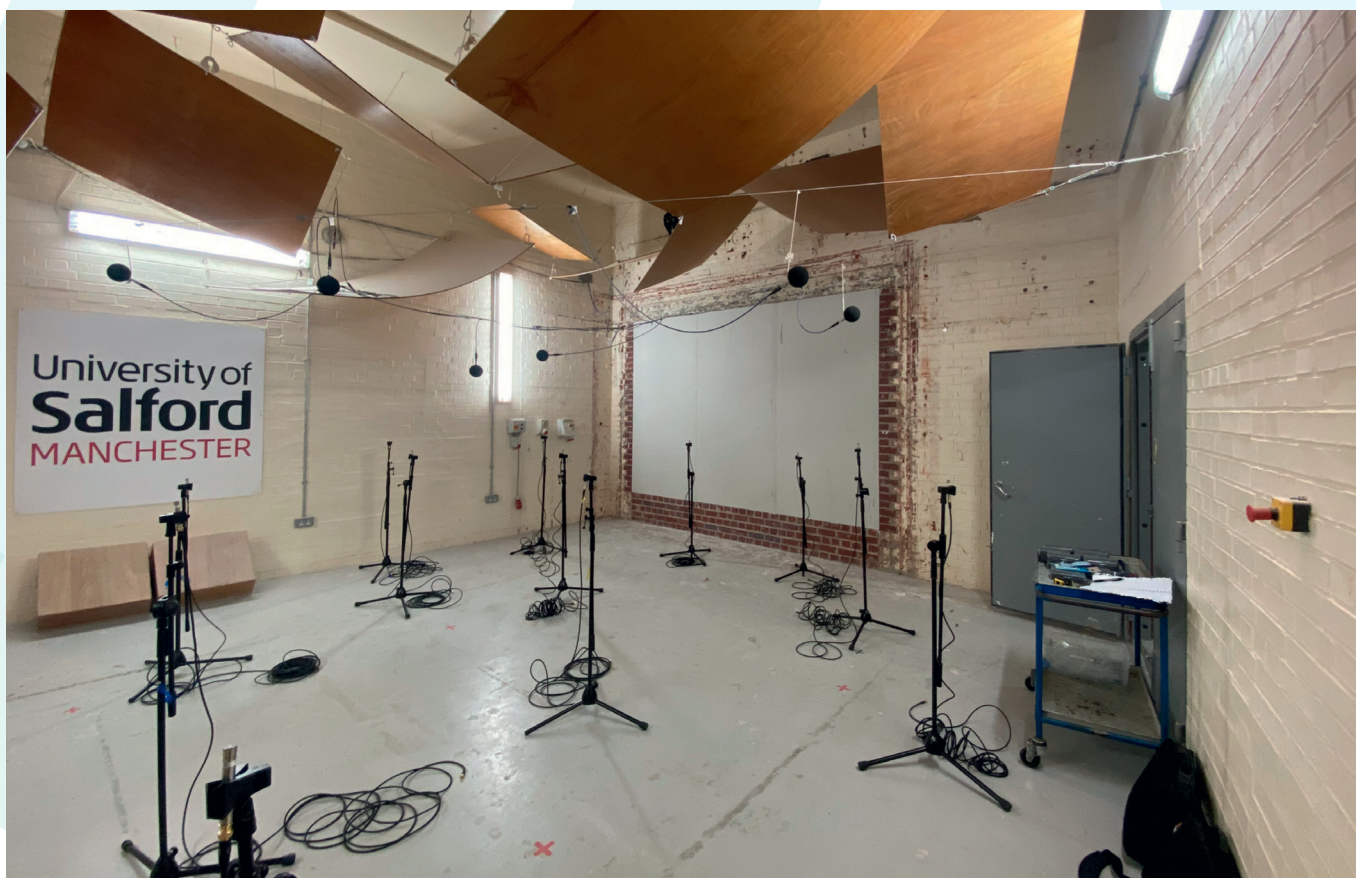
Above: Microphones positioned randomly in the receiving room at the University of Salford. Plasterboard partition located in aperture
