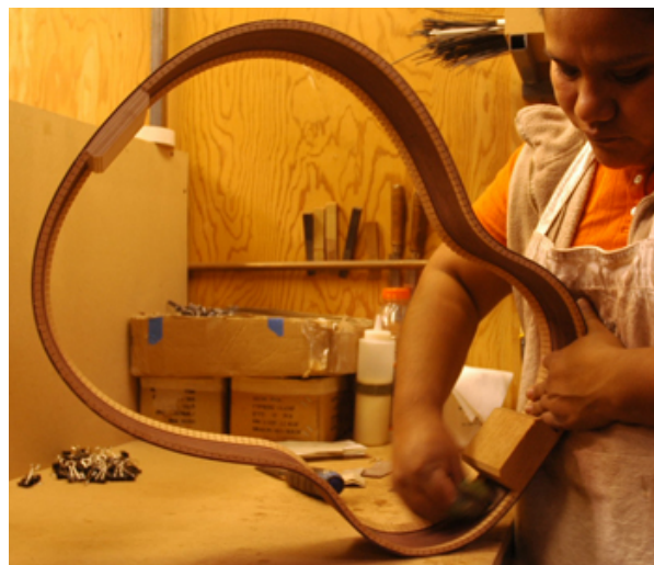
The inner part of a guitar frame is meticulously sanded to remove any surface imperfections, despite the fact that the final result will be hidden when the guitar is fully constructed.
