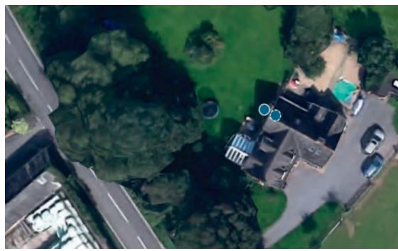
Left: Measurement positions 1.5m from glazing, 1.5m above the ground either side of the window. Meters located central to the window
