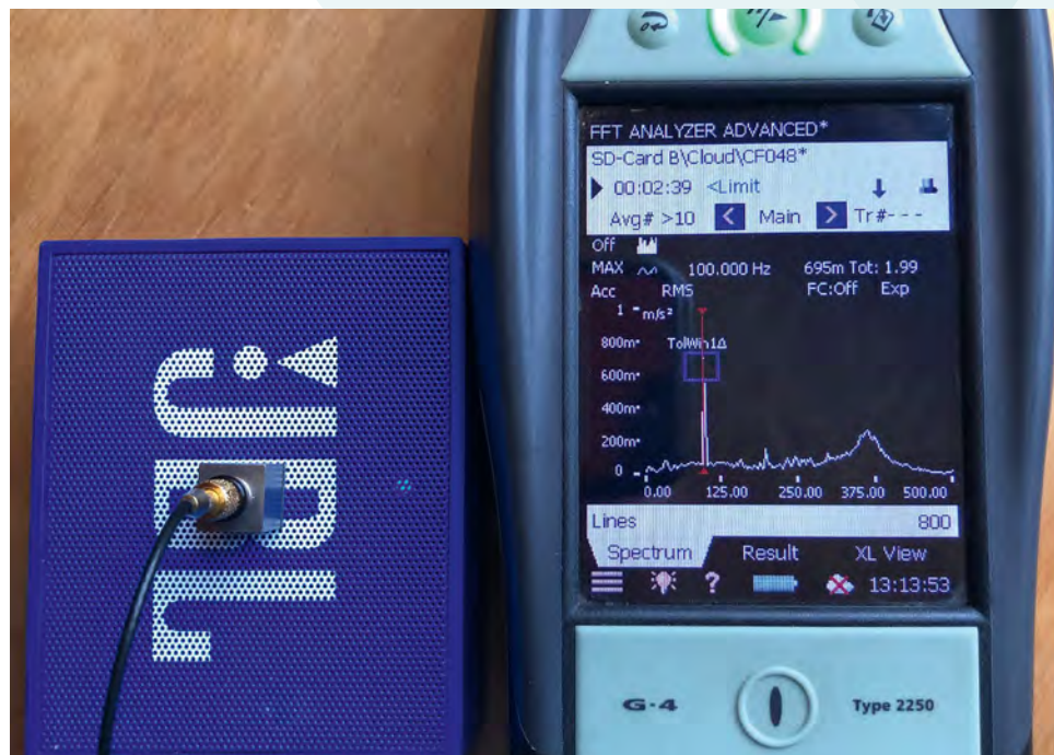
Below: Figure 1: Accelerometer on Bluetooth speaker measuring 100Hz Tone
