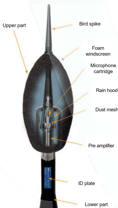
Above: Figure 4: Typical weather protection for class 1 measurement microphone system
