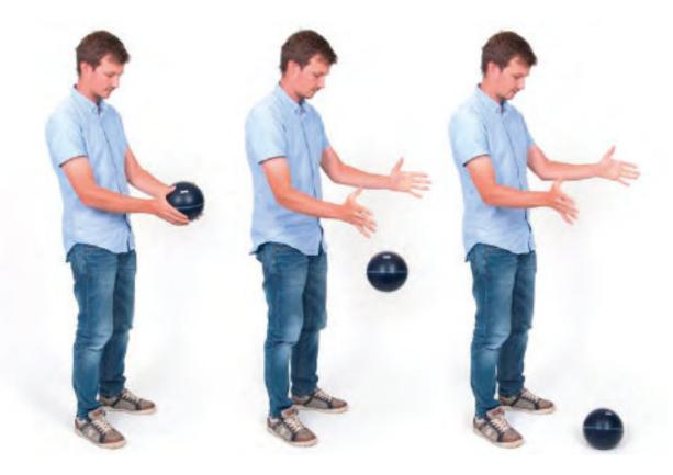
The tapping machine requires the use of an energy-averaged sound pressure level, whereas the rubber ball uses the maximum sound pressure level measured with a fast time weighting and energy averaged across each source position. The methods used for measuring the reverberation time of the receiving room are identical for both the tapping machine and the rubber ball.
