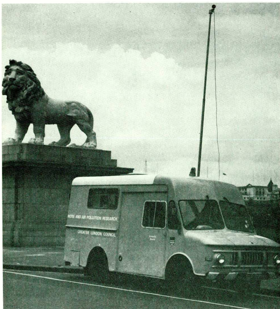
Early type mobile laboratory, with pneumatic mast
