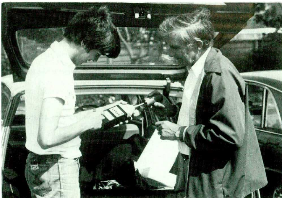
For accurate noise measurements a calibrated sound-level meter and sound calibrator are required
