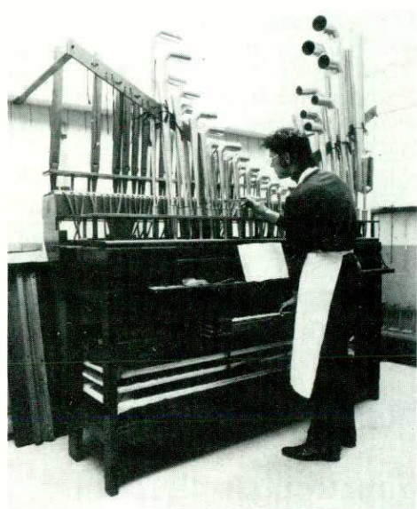
Figure 5 Voicing machine — a small single manual organ
