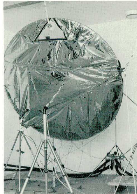
Fig. 3. Satellite antenna prepared for testing in the large reverberation chamber.
