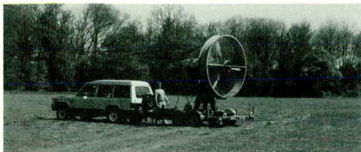
Fig. 17. Cabin noise transmission loss rig; mobile propeller unit for noise propagation tests
