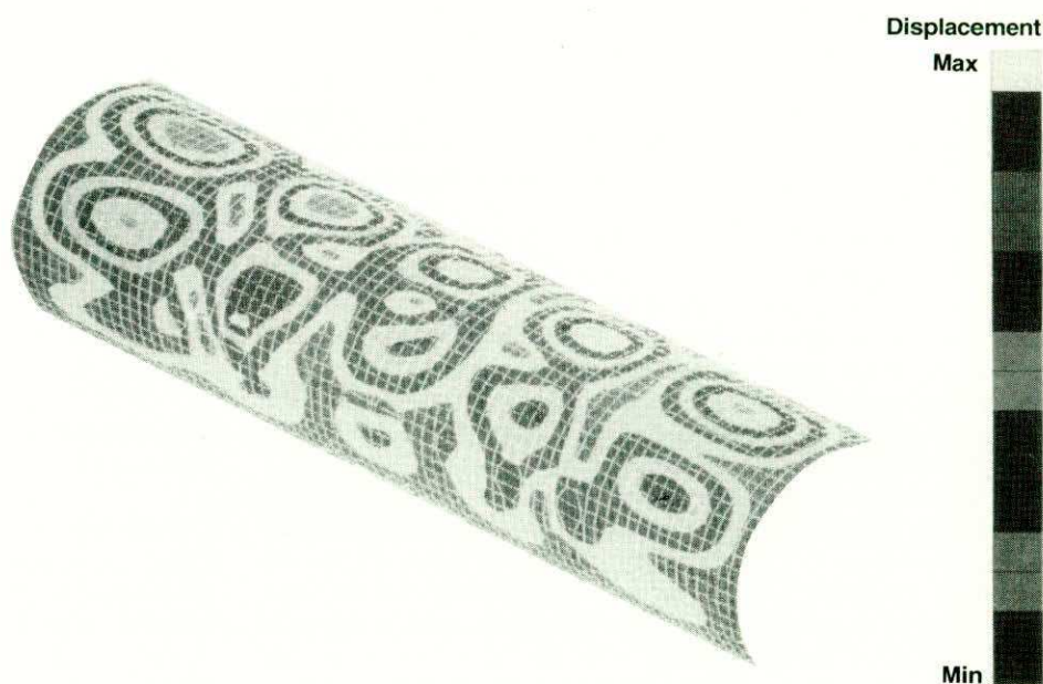
Fig. 21. Cabin noise prediction: typical structural response
