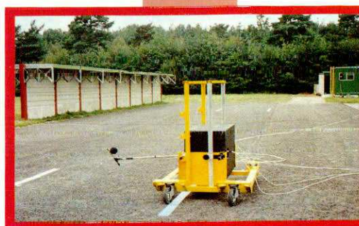
Measuring the acoustic performance of 'T' shaped barrier using the Barrier Test Facility at TRL
