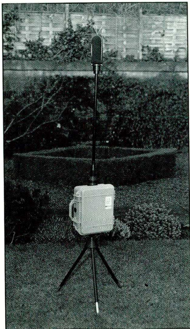
CRL 245 Portable Noise Logger
