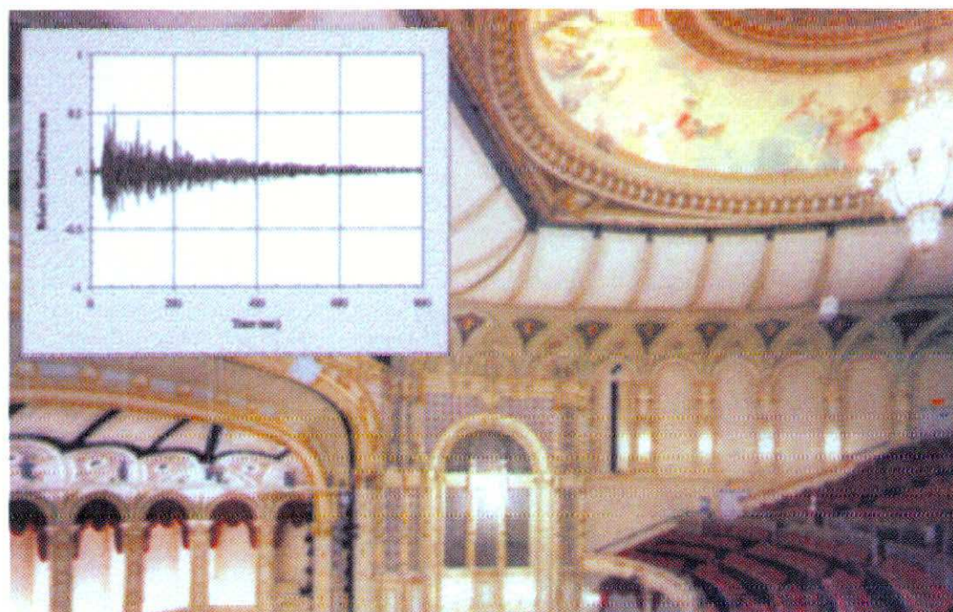
Fig. 2 After the renovations, the impulse response demonstrates the ideal 'Christmas Tree' configuration.
