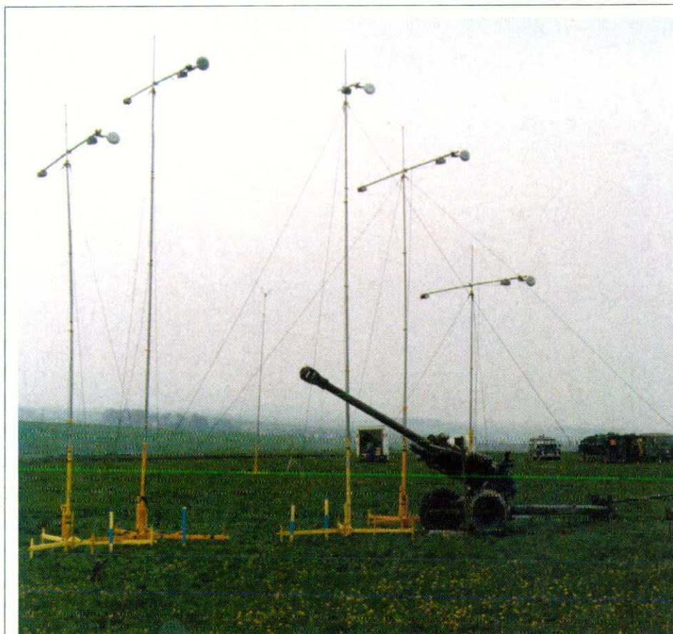
Measuring source levels of guns
