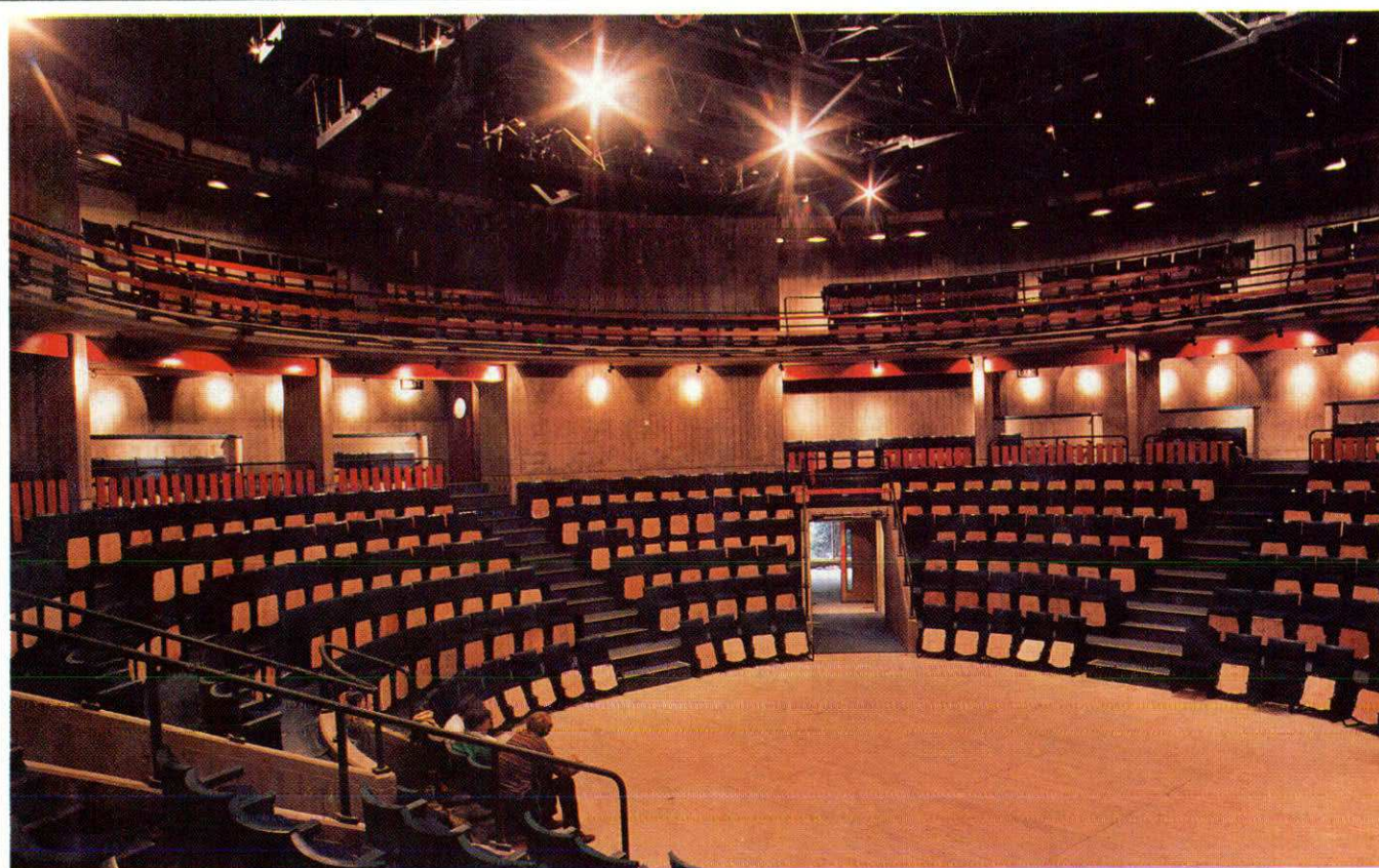
Fig. 3. The design of the New Victoria Theatre, Stoke on Trent, was one of the earliest applications of Rupert Taylor's ray tracing software. The geometric shape of the reflectors suspended above the stage area of the theatre-in-the-round was designed to maximise early reflections from each performer around the full 360° auditorium.
