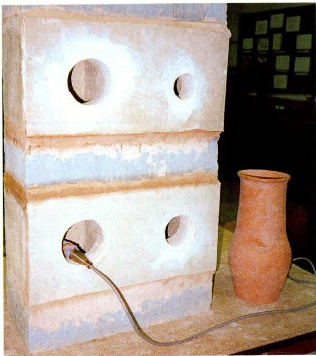
Fig. 4. The testing arrangement for resonators cut into hollow blocks showing a microphone in place for testing. One of the Russian pots is seen alongside.
