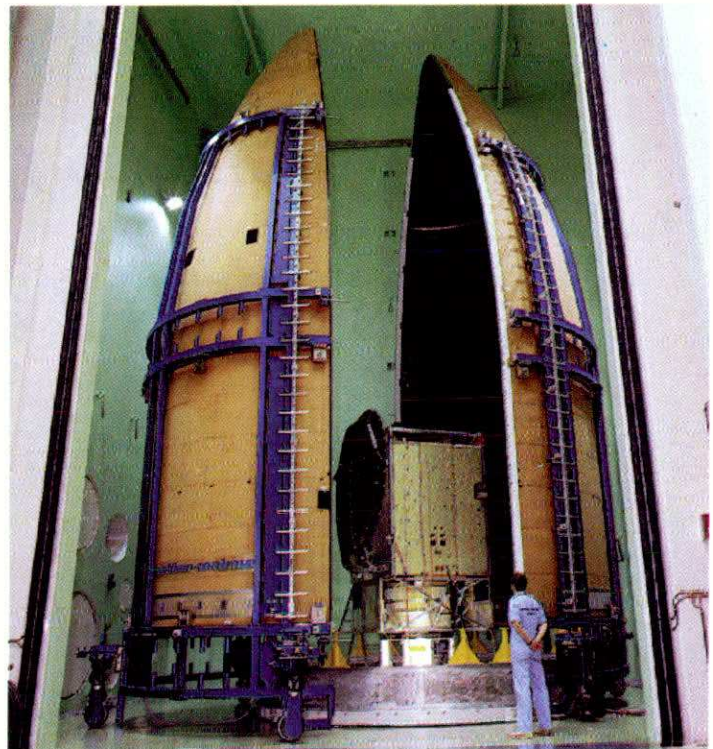
Fig. 5. DASA-Dornier (D) and Oerlikon-Contraves (CH) successfully developed the Ariane-5 fairing with its passive noise-control system, shown here with the Olympus test structure used to assess acoustic performance in the LEAF
