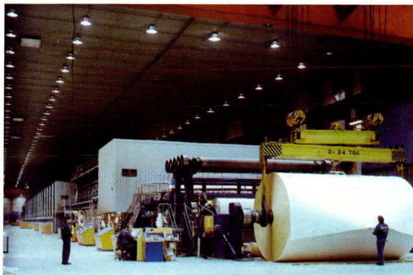
Modern paper machine; the size of machine and paper rolls is impressive
