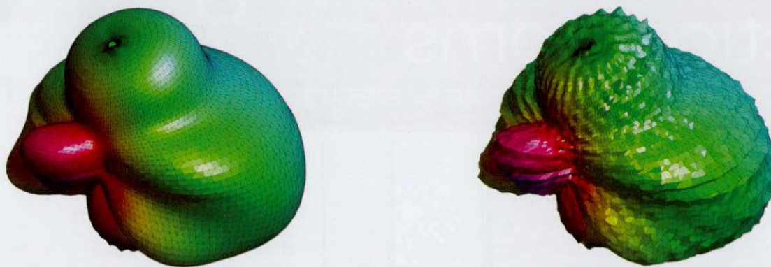
Figure 5. Balloon plot of an HRTF at 1 kHz (left) and its simulation by the spherical loudspeaker array (right).
