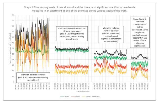
At several sites it became apparent that the issue of ground loop pipe coupling to the floor was significant and we advised that the concrete around the pipes should be broken out (by others). This work was also undertaken while the systems remained in operation and was successful in achieving further reductions of varying significance at different premises. This also allowed yet further reductions to be achieved by adjustments and refinements to the other isolating elements.
