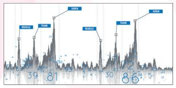
To help identify the cause of a noise level alarm, NoiseScout now provides a text description of the content of the wav files that are recorded during an alarm event. This is achieved using AI analysis and noise classification.
