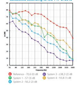
**AIRBONE NOISE RESULTS** Calculated according to ISO 717-1: 2013
