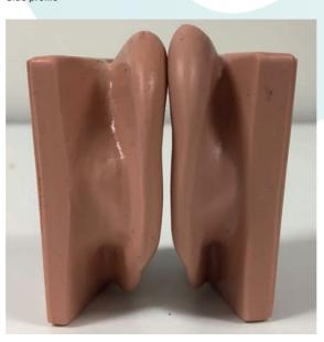
which utilises pinnae that are not symmetrical as they are based on real measurements of human dimensions. Figure 1 and Figure 2 show the pinnae used for this project and provide clear evidence of the differences that will lead to decorrelation of not only the reverberant field but also the direct sound source.
