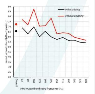
Figure 8 shows a reduction of around 5 dB in most frequency bands, but a significant reduction in the previous peaks at around 100 and 200 Hz.
