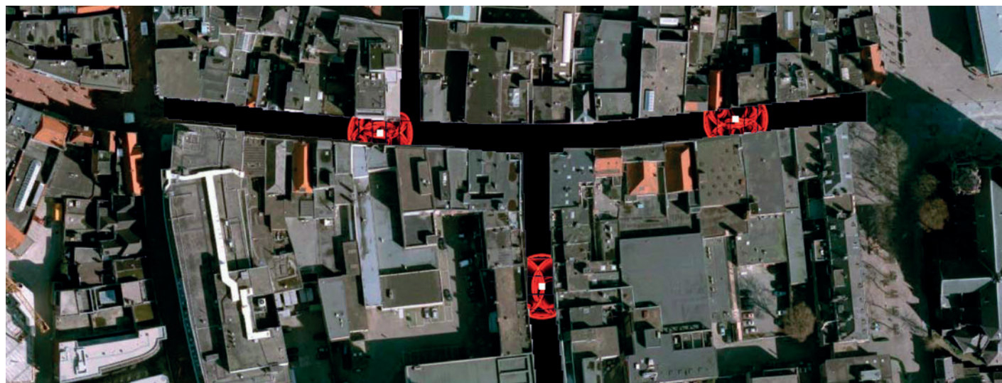
More precise models of how sound waves travel as they bounce off buildings in cities could help urban planners come up with more targeted solutions. Image courtesy of openPSTD.
