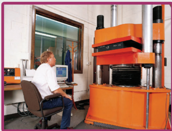
Bearing Testing at Mason Industries HQ
