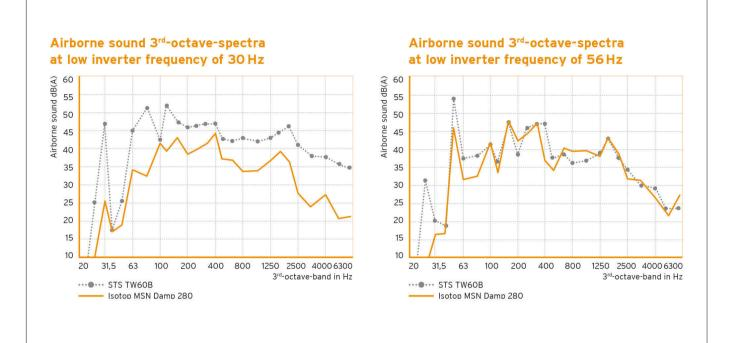
improvement in the critical low-frequency range is achieved with Isotop MSN-DAMP. At low rotational compressor speeds of 30 Hz, there is a significant reduction in sound radiation over the entire frequency spectrum; at higher rotational speeds there is a drastic improvement, especially in low-frequency ranges (see Figure 5).
