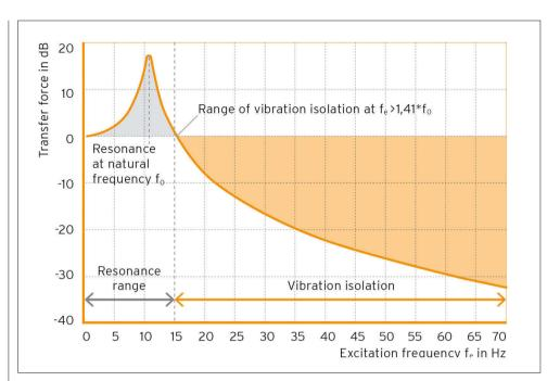
Above: Figure 2: The isolating effect occurs if the ratio of excitation frequency to natural frequency is greater than  $\sqrt{2}$  Elastic components made from polyurethane are ideal for meeting the ever-increasing demand for the reduction of vibrationinduced sound radiation. Their excellent dynamic properties are advantageous compared to rubbermetal elements.
