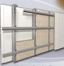
New metal stud wall 2 layers of 15mm sound grade plasterboard, 70mm metal stud frame, 50mm insulation, *Isoblock & Isobar*,
