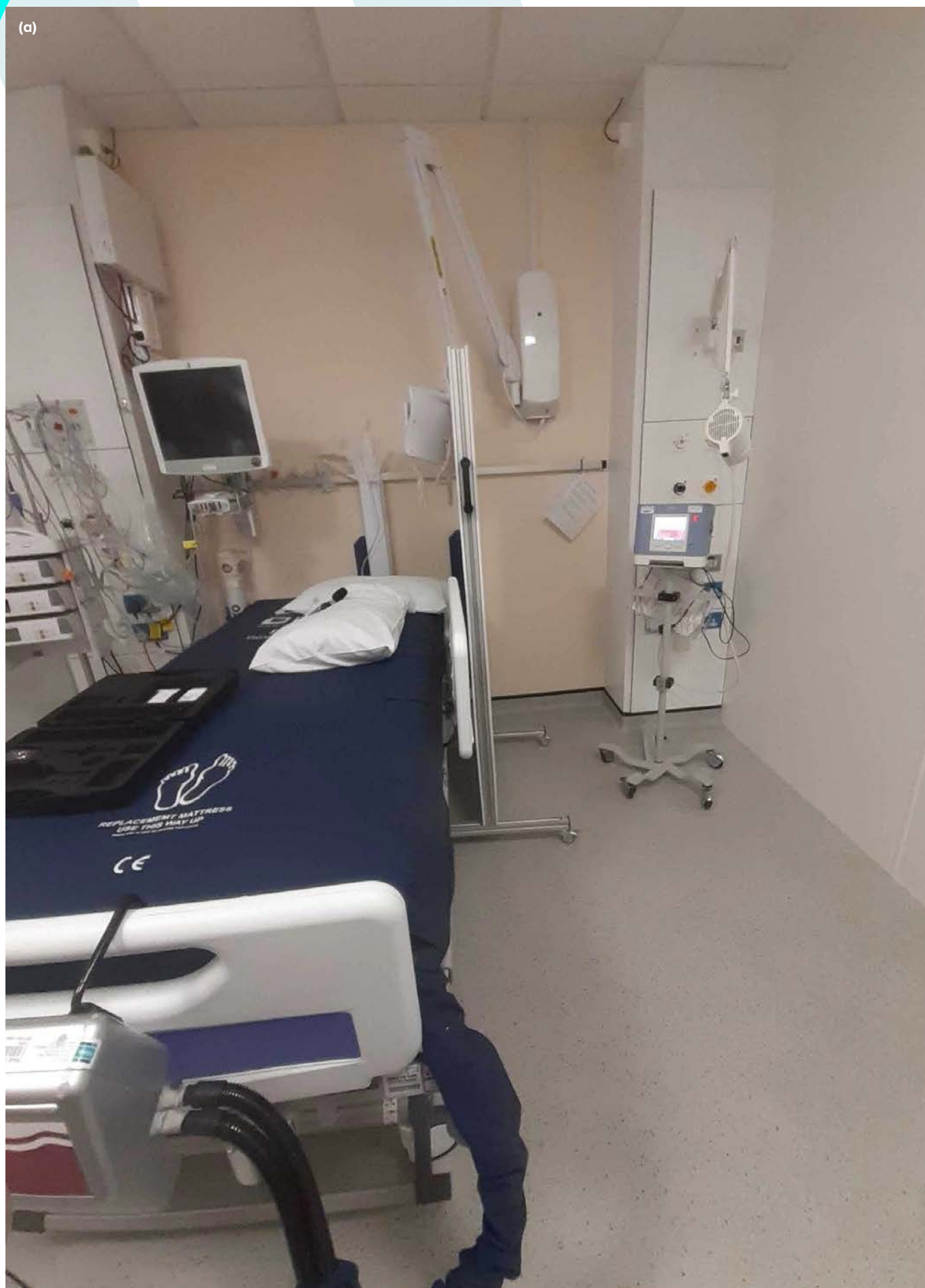
Above and right: Figure 6: Testing in situ: (a) the movable barrier positioned between the bed and the equipment, in the position labelled as 'close to the bed' and (b) the measurement equipment (on page 55)
