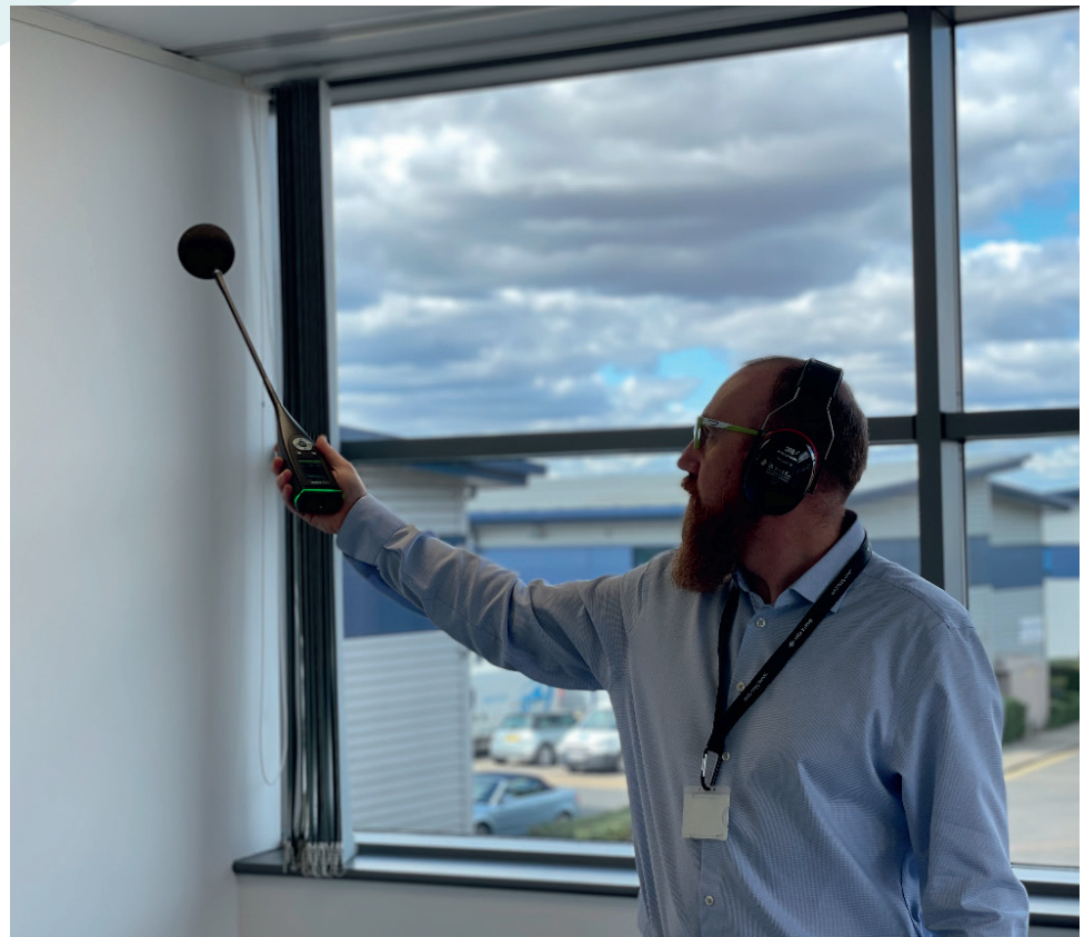
Above: Figure 6: Moving microphone method with extension rod
