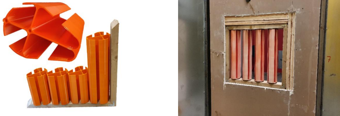
Figure 6 3D prototype of the final profile. Left: sectional view, Right: Installed within test rig. Ref [8]
