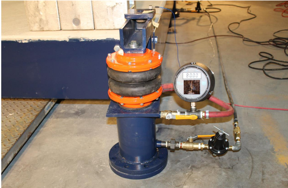
Figure 6 – Close up of air spring. The accelerometer can be seen on the top of the spring bracket.
