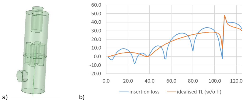
Figure 4: a) CAD schematic of the existing silencer; b) predicted transmission loss and insertion loss of the existing silencer system.
