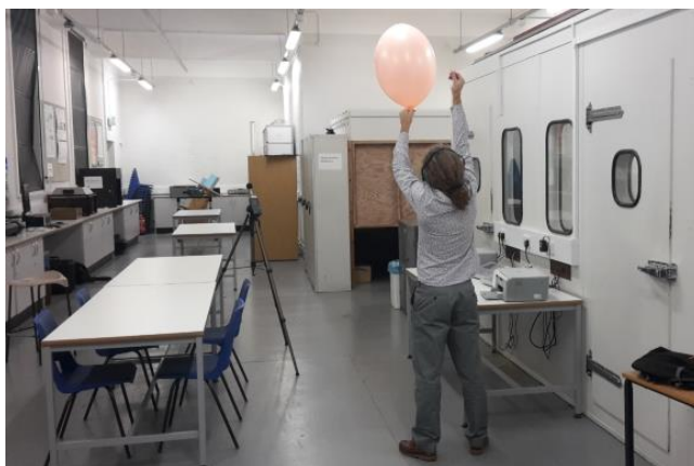
Figure 1. Balloon pop being used to obtain an impulse response of the LSBU acoustics laboratory
