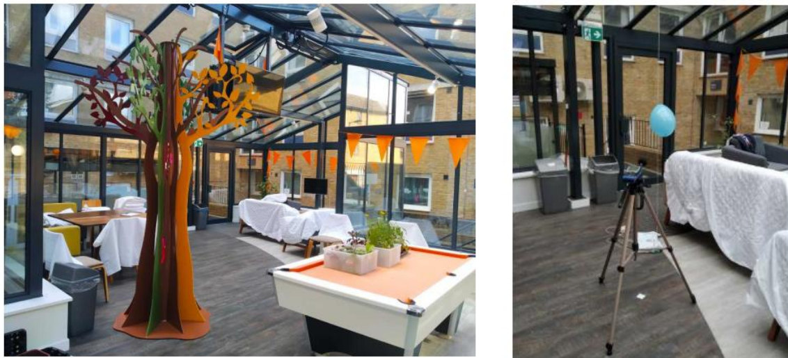
Figure 2. Left: room used; Right: balloon sample in position and sound level meter at 3m away
