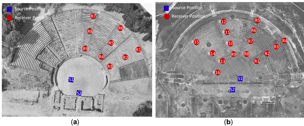
Figure 2. Scheme of the equipment positions assumed during the acoustic measurements: in Tyndaris (a) and Volterra (b).
