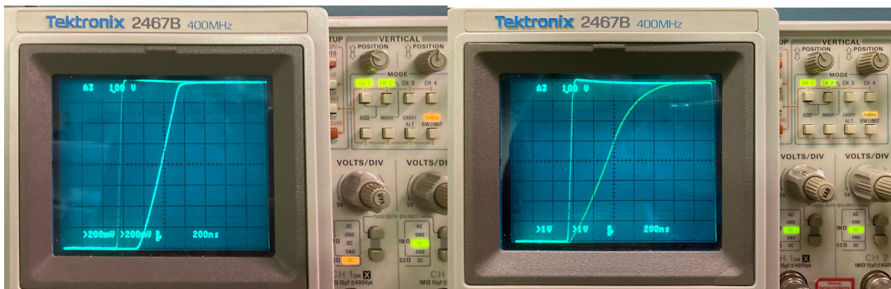
Figure 6: Oscilloscope traces of square-wave signals introduced to a G.R.A.S. Type 26AB microphone pre-amplifier connected to the G.R.A.S. Power Module set to +20 and 0 dB gain, respectively. In both oscilloscope images, the left trace is the rising edge of the reference 350-kilohertz square-wave signal and the right trace is the corresponding output from the Power Module. The left image shows a 400-nanosecond rise time for an output signal of 2.4 volts peak-to-peak (50-ohm load). The right image shows a 700-nanosecond rise time for an output signal of 8.6 volts peak-to-peak (one-megohm load). The initial slew rates are 6 and 13 volts per microsecond, respectively. With respect to the left image, the initial 200-nanosecond delay for the output signal is caused by a 30-meter microphone extension cable that was temporarily inserted between the pre-amplifier and the Power Module.
