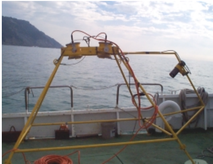
FIGURE 9. Underwater components of the digital stereo camera system. The cameras are housed in the containers at the top of the frame and a high-intensity strobe is seen at right.
