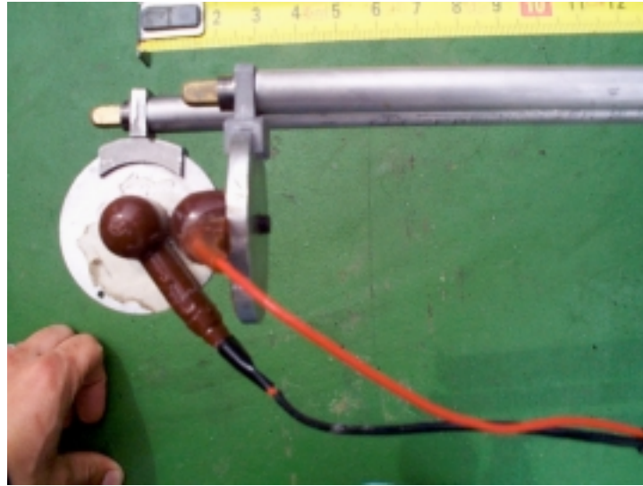
FIGURE 16. Pair of uni-axial accelerometers mounted to coupling disks. The sensors are attached to a burial jig using clips on the edges of the disks. Springs temporarily fix the clips to the inner, square, rod of the burial jig. The sensors are released when the rod is retracted.
