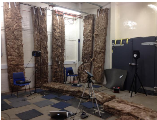
Figure 1 The reverberation chamber showing the measurement setup including absorption, T_{60}=0.4 s
