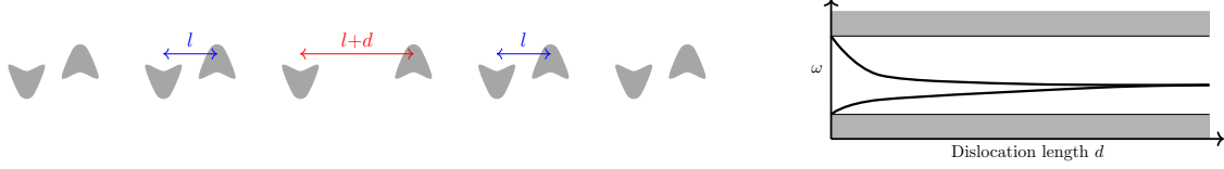
Figure 4: Introducing a dislocation to the three-dimensional SSH structure causes two topologically protected mid-gap modes to be introduced at either end of the dislocation. Their eigenfrequencies appear at either side of the band gap and converge on a single position within the band gap as the dislocation becomes arbitrarily large.
