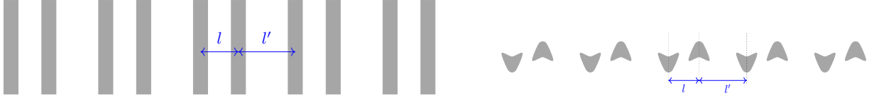
Figure 1: The two SSH-type metamaterials that we will consider in this work. Left: a sequence of lamina, arranged in an SSH-type pattern, which we study using high-frequency homogenisation. Right: an array of three-dimensional bounded material inclusions arranged according to an SSH-type pattern in one dimension, which we study under a high-contrast assumption. In both cases, the lengths l and l' are the crucial parameters which describe the materials' topological wave transmission properties. The materials are periodic with periodicity length L = l + l' .
