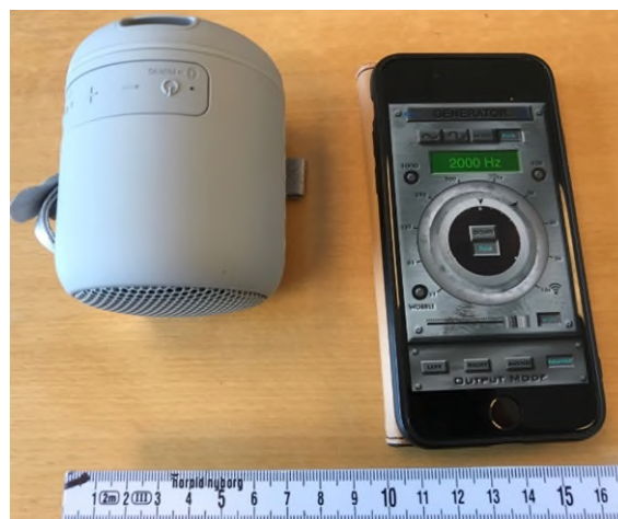
Figure 1: Simple and cheap noise source using Bluetooth connection from App noise generator.
