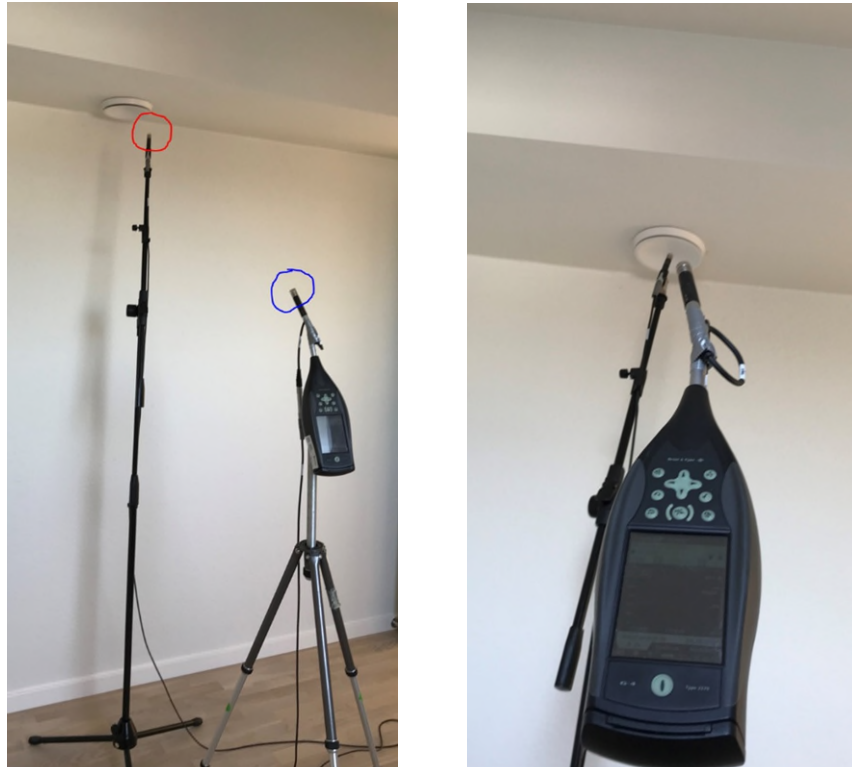
Figure 6: Setup in room B. Armature downward, near wall. Right picture shows the alignment of microphones pointing at center of armature.
