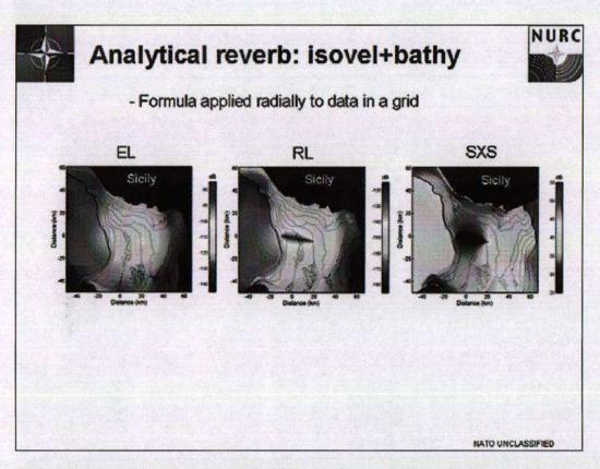
36 I've already mentioned some analytical formulae for reverberation. Those were for parametrised environments, ie shelf depth, bottom slope, etc. It's also possible to operate these formulae for bistatic sonar along radials from the source and receiver, but you insert effective depths calculated from a grid. This is target echo, reverberation, and signal-to-reverb-ratio between Sicily and Malta. The whole lot takes a couple of seconds on a PC.
