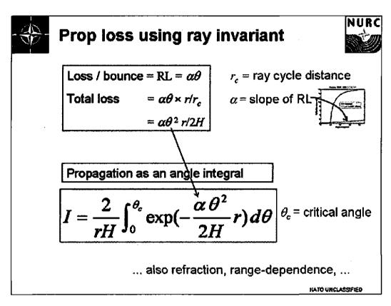
15 What can you get with this? Well you can bung it into a formula and get propagation loss, and this can be extended to range-dependent environments, refraction, and so on.
