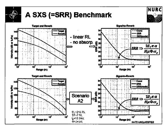
31 To make this a bit more quantitative and pertinent to this workshop's Test Cases I can put this all into an analytical model.
