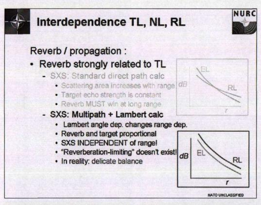
30 ... but if you take account of the way the scattering law depends on angle – for instance Lambert's law – you find that the increase in area is exactly compensated by this and the reverberation and target echo decay in parallel. So reverberation limiting doesn't exist. Instead you have noise limiting.
