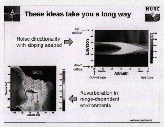
16 Using these ideas you can get a long way, not just with propagation, but with ambient noise, reverberation, and signal excess.
