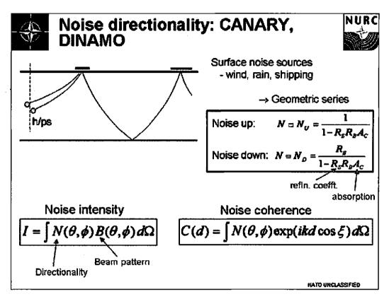
35 CANARY and DINAMO are noise models. CANARY was a research model that calculated noise directionality and noise coherence for all sorts of arrays, including conformal ones. DINAMO calculated noise levels as a function of locality. I think it got used on UK submarines.
