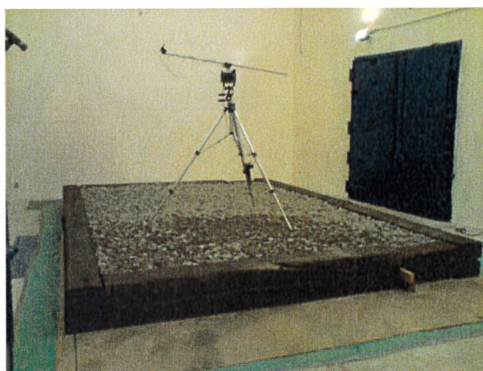
Figure 7. Measurement of diffuse incidence absorption coefficients of railway ballast in a reverberation room. Results are shown for two different thicknesses. 24
