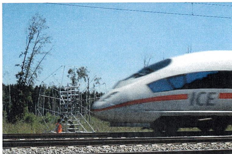
Figure 13. Microphone array with 4 m diameter in use to separate noise sources on a moving train.
