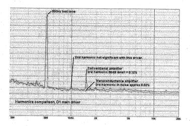
The above plot shows a spectrum analysis from a driver being driven normally with a 500Hz test tone. The blue line shows the result when driven with a normal voltage mode amplifier. The green line shows the response when driven with the same amplifier, operating in a transconductance implementation (with current sensing feedback).
