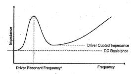
The impedance of the driver changes with frequency. But there is much more still to (Z). A more complete equation to relate the force on the loudspeaker driver cone is:
