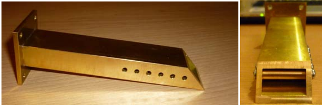
Figure 3: First attempt to produce a bioinspired antenna using a waveguide. This device had limited success due to the differing fundamental modes of the acoustic and electromagnetic waveguide.
