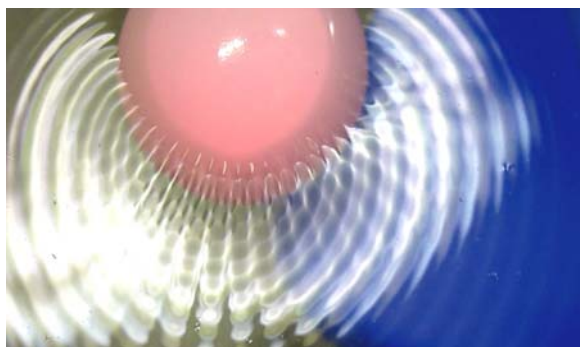
Figure 8. Scattering, radiation and strong interactions of a vibrating HSD, Elmer et.al. (2011) 8 .
