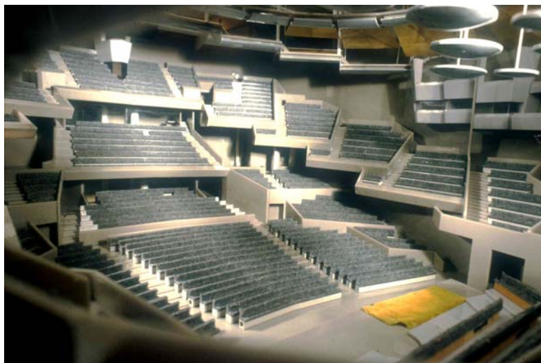
Figure 4. View of the interior of the 1:50 scale acoustic model of the Waterfront Hall, Belfast
