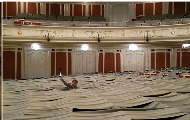
Figure 15. Stalls with audience simulation (curtains) and one of the authors with a sound level meter.
