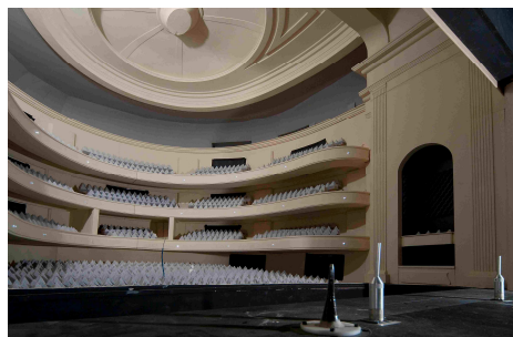
Figure 6. Scale model 1:10 with the raised ceiling and reverberation gallery. High frequency source and microphone with pre-amplifier in foreground.
