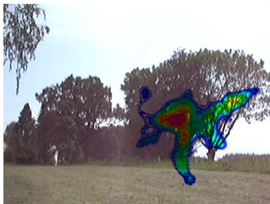
Fig. 5 The acoustic camera; frequency range > 2000 Hz
