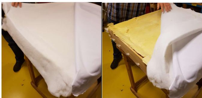
Figure 8 Second mineral wool top layer of rockwool (25 mm, 45 kg/m 3 ) and foil underneath
