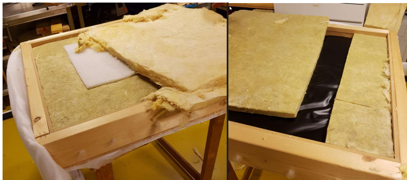
Figure 8 Second mineral wool top layer of rockwool (25 mm, 45 kg/m 3 ) and foil underneath
