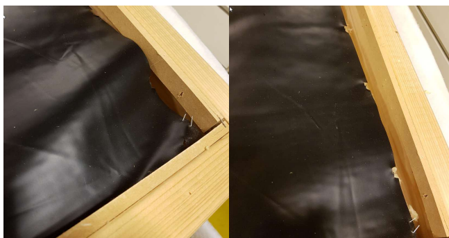
Figure 9: pvc-foil (650 g/m 2 ) mounted from the back with staples, but clearly loosened from the (top) side.
