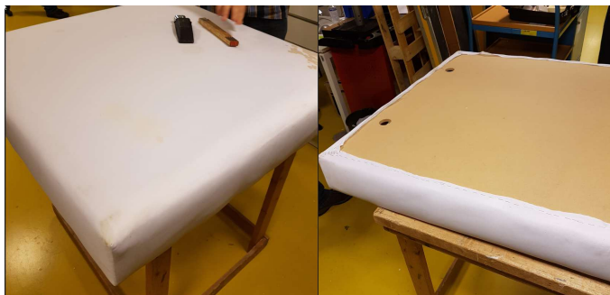
Figure 5 Front view and back view of cushions (with 2 holes in back panel for hanging of wall panels)
