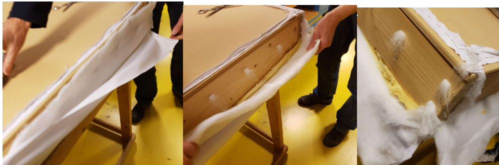
Figure 7 Top side with textile finishing, additional fleece layer and top layer of glass wool (40 mm, 22 kg/m 3 )
