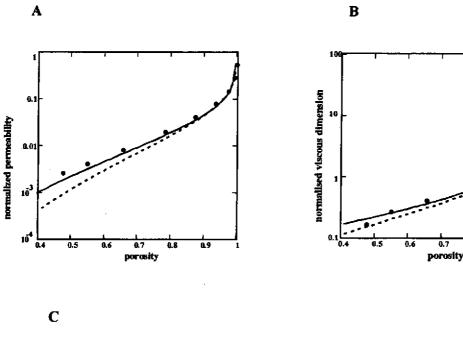
Figure 1. Dimensionless DC permeability  $\frac{k_0}{d^2}$  ( $d=\sqrt[3]{\frac{4\pi}{3(1-\phi)}}R$  is the base vector of the lattice) (A), characteristic viscous dimension  $\frac{\Lambda}{d}$  (B) and formation factor  $F=\frac{\alpha_{\infty}}{\phi}$  (C) for SC packing as a function of porosity, circles – numerical results [9], solid line – cell model (10), dashed lines – cell model (9).
