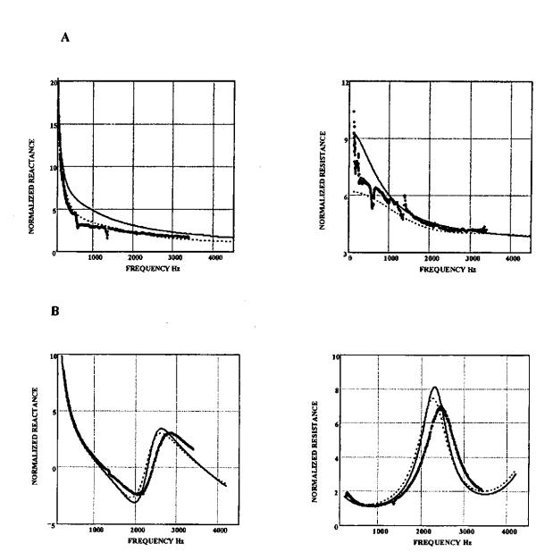
Figure 2. Comparison between predictions of normal surface impedance for a layer of glass beads and impedance tube data. Porosity is 0.39, calculated value of tortuosity is 1.78, layer thickness is 0.0475m, mean bead radius is either  $5.625 \times 10^{-4} m$  (A) or  $1.7 \times 10^{-4} m$  (B), measured value of flow resistivity is either 13400mks rayls/m (A) or 240000mks rayls/m (B). Solid line – modified characteristic dimension model, dashed lines – cell model.
